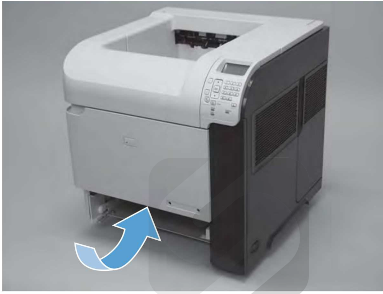
Figure 2-7 Remove the Tray 2 separation, pickup, and feed rollers (3 of 4)
