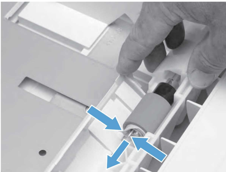
Figure 2-6 Remove the Tray 2 separation, pickup, and feed rollers (2 of 4)
