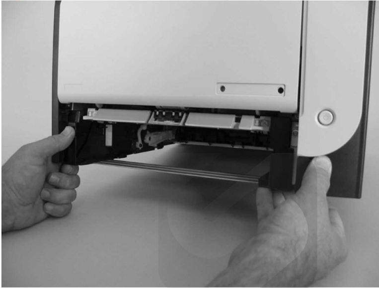
Figure 6-4 Remove the pickup roller (1 of 2)
